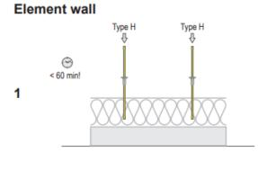
Fill in and compact the concrete of the first shell. Apply the insulation as tightly as possible to the fresh concrete of the first shell. Insert Thermo-Pins through the insulation into the fresh concrete of the facing layer.
