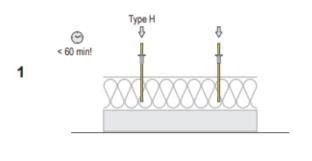
Fill in and compact the concrete of the first shell. Apply the insulation as tightly as possible to the fresh concrete of the first shell. Insert Thermo-Pins through the insulation layer into the fresh concrete of the facing layer.
