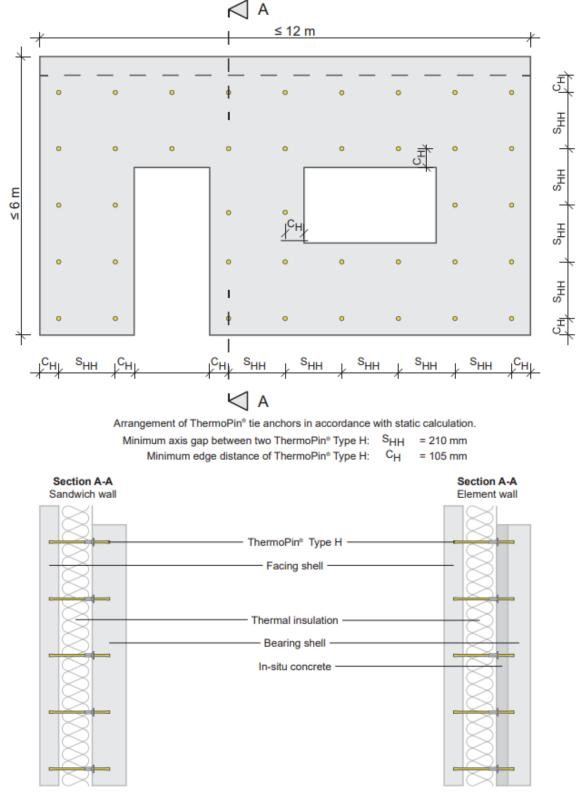
Arrangement of ThermoPin® tie anchors in accordance with static calculation.
