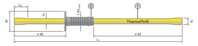
ThermoPin° tie anchor Type H: GFK anchor with straight plastic sleeve. Dimensions in [mm].
