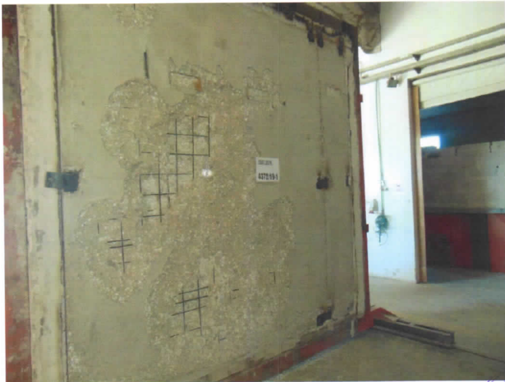
Photo 10: Specimen on the side exposed to fire after testing
