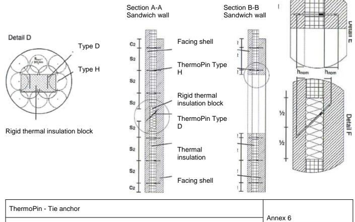
Assembly parameters and thickness of shell
