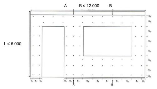
Arrangement of ThermoPin tie anchors in accordance with static calculation. Standard gap between ThermoPin tie anchors Type H: s = 300 - 500 mm. Standard edge distance: c = 150 - 200 mm.
