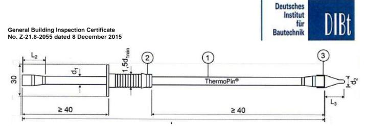
ThermoPin tie anchor Type H: GFK anchor with straight plastic sleeve. Dimensions in [mm]
