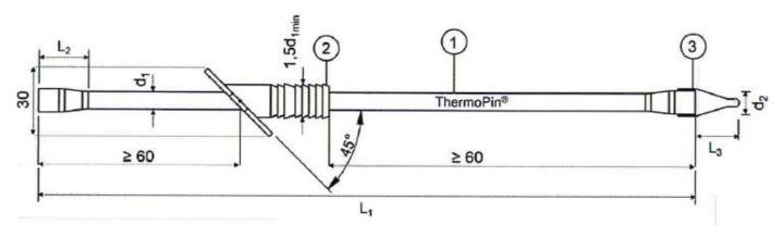
ThermoPin tie anchor Type D: GFK anchor with sloping plastic sleeve. Dimensions in [mm]
