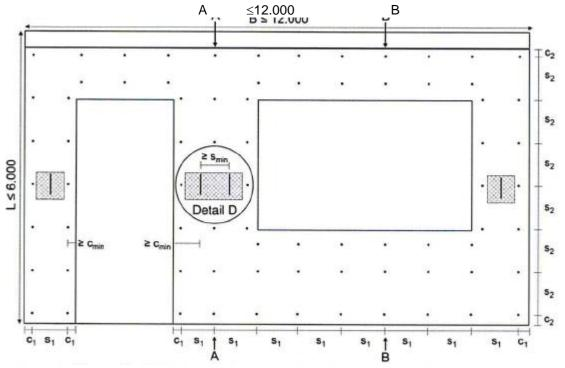
Arrangement of ThermoPin tie anchors in accordance with static calculation. Standard axis distance of anchors Type H and Type D: s = 300 - 500 mm. Standard edge distance: c = 150 - 250 mm.
